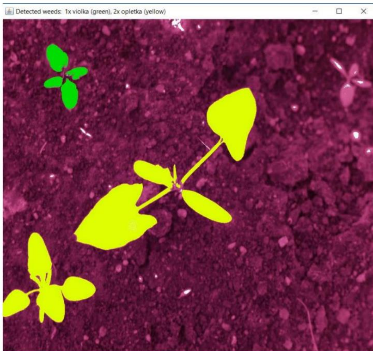
Figure 2: Detection of individual weed species: sample use in a GUI application
